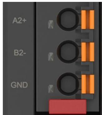
使用双绞线连接至 A 端子和 B 端子，双绞线的另一端分别连接到对端设备串口的 RS485+ 和 RS485- 端子即可。Use twisted pair wire to connect to A and B terminals, and the other end of twisted pair to RS485 + and RS485- terminals to the serial port of the peer device, respectively.
